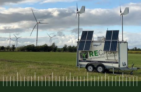
LiDAR wind measurement system
